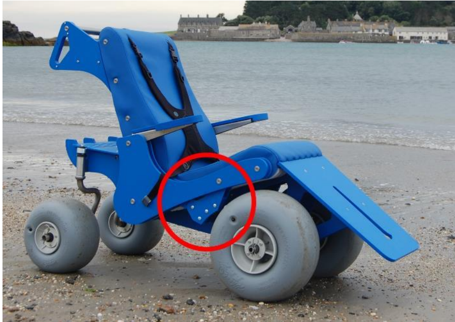
Figure 6: Sand chair prototype using HDPE plastic (brake assembly circled)
