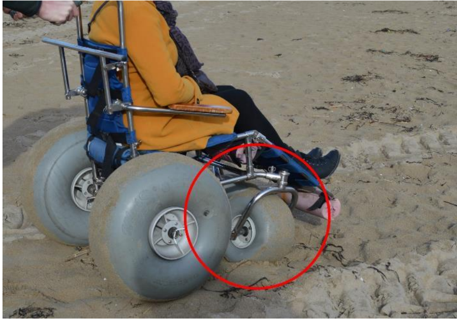
Figure 1: Landeez™ front wheels snagging in the sand
