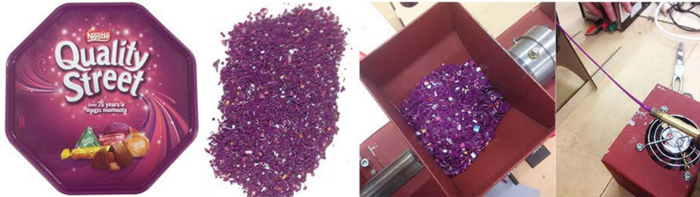
Image ©Co-product CIC 2015. PP Quality Street Packaging: shredding, filament extrusion and initial 3D print tests.
