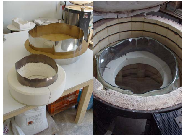
Figure 9. The process of developing the glass shapes.
