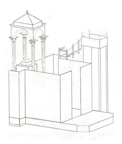
This final drawing uses the space of the enclosure entrance and step. This drawing uses parallel projection, and therefore does not use any vanishing points, all the lines from a given face are parallel to each other.
